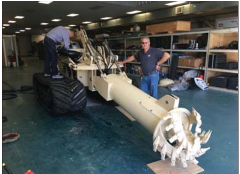
The MRSD came equipped with a cutterhead (shown here) but the Corps has been testing the unit with different types of heads to further expand how the dredge can be used.
