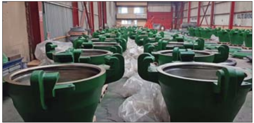
Dredge ball joints are used as a flexible connection or coupling between steel pipelines.
