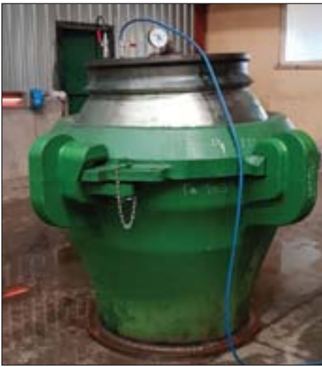
Dredge ball joints are used as a flexible connection or coupling between steel pipelines.
