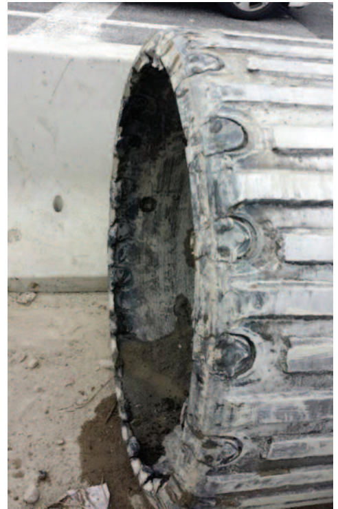
Worn Out Starter – It was not uncommon to have to rebuild a segmented double wall starter casing after drilling one hole.
